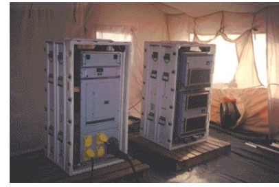
Tactical weather radar system- Complete fully coherent C-band system, including antenna and tower, packaged on one standard air freight pallet, fits in C130 type aircraft. Setup by 2 person crew with no additional equipment. Only shelter and electrical power required.
