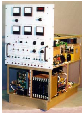
Military 1 MW C-Band Transmitter (Currently being FCC Type Certified for commercial sale in the U.S.)
