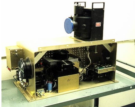
1 MW S-band Transmitter Module Including Solid State IGBT Modulator
